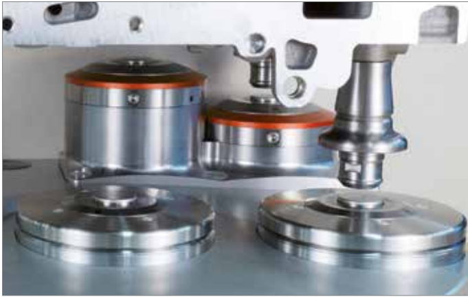
Workpiece with multiple clamping and support points
