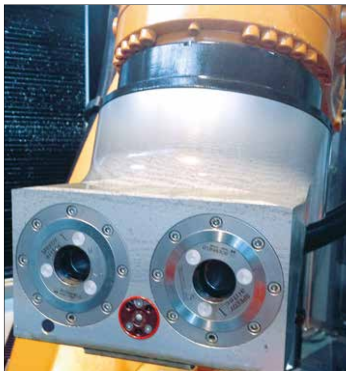
Example: Gripper for robot with pneumatic and electrical coupling
