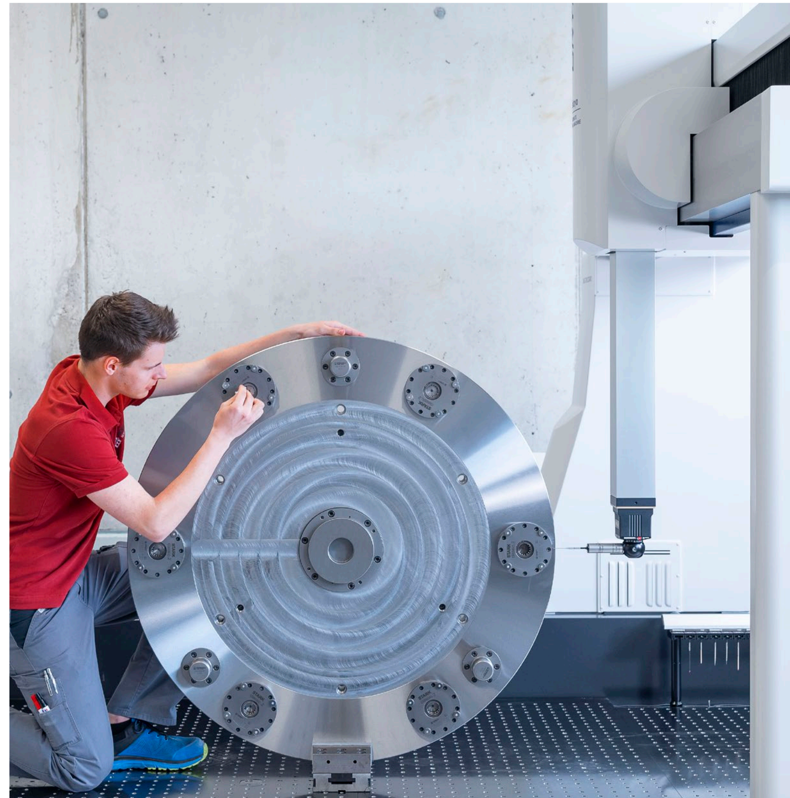
Quality checks are carried out in an air-conditioned measuring room. Customised fast clamping locking plate with a diameter of 1.1 m for grinding applications in the aviation sector
