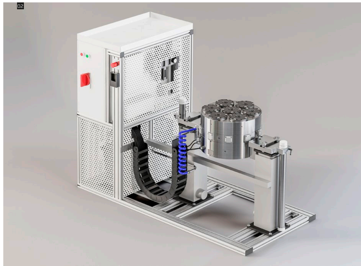
01 STARK robot gripper with a zero point clamping system enables automated pallet changes even without media on the machine table. Media transfer for clamping and release processes as well as necessary control queries take place via a multiple coupling on the pallet gripper. This system is also ideally suited for retrofitting projects.
