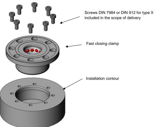
1. Check the installation contour for the STARK.basic for dimensional accuracy and surface quality. Important: The transition from the insertion chamfer to the centring bore must be burr-free, otherwise the O-ring may be damaged (leakage and failure of the fast closing clamp). All parts must be clean, this also applies to all supply lines. (deep-vores, pipes, hoses, etc.).
